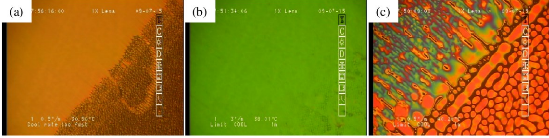
Fig.3.2 The polarized microscopic images of the LC mixture of 8CB and 7CB ( \phi=10.2 wt%) at 30.5 °C (a), 38.0 °C (b) and 40.4 °C (c) on heating.
