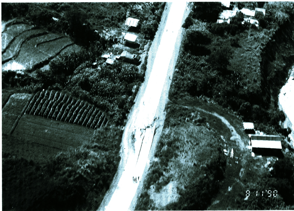
Photo 2. Aerial view toward the east showing offset of the Digdig fault 500 m north of the point shown in Photo 1.
