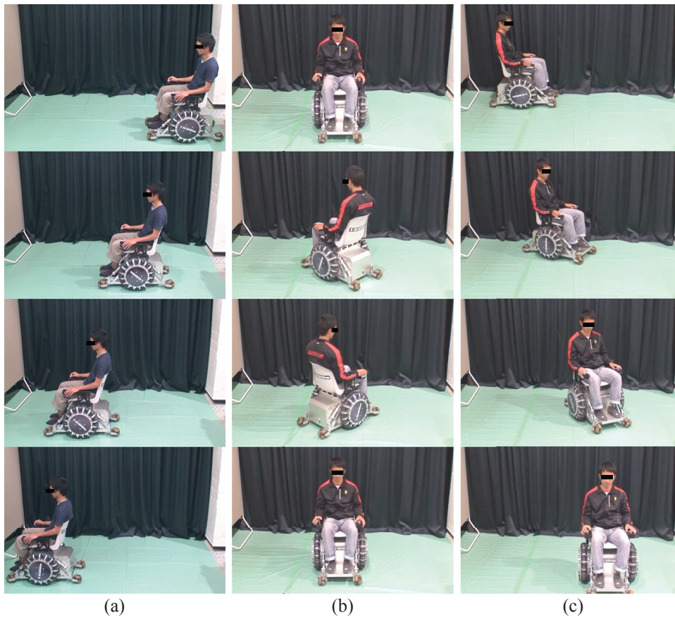
Fig. 5.11 Motion in the longitudinal movement mode. (a) Forward translation. (b) Spin turn. (c) Forward translation with right spin.
