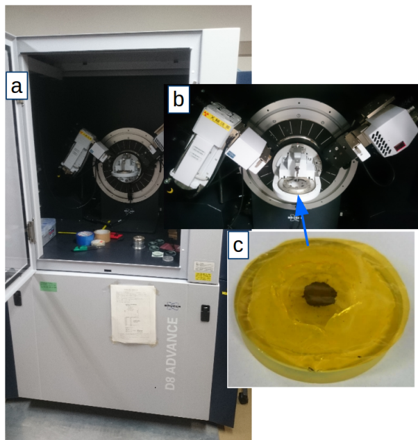
Figure 3.1: (a) Bruker AXS, D8 Advance used for XRD diffraction experiment. (b) The X-ray source on the left and detector on the right, and sample holder goes in the middle. (c) Typical glass sample holder setup for air sensitive samples with powdered sample in middle (black), Kapton sheet on top, and vacuum grease between the glass and the Kapton sheet.
