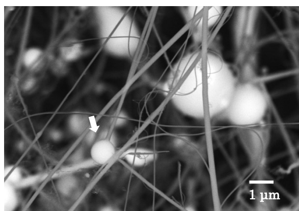
Fig. 2 SEM image of the generated nanofibers. The arrow points a tip of nanofibers.
