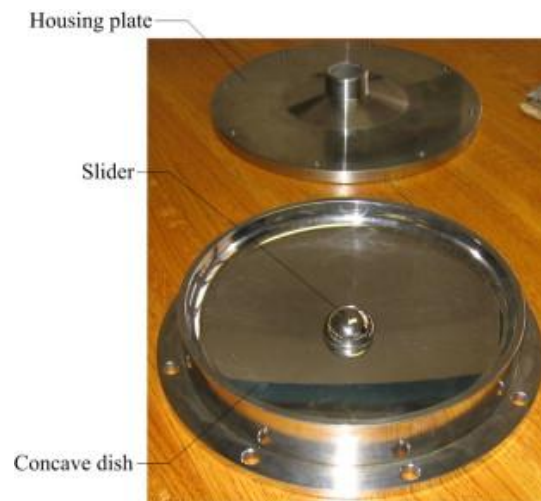
Figure 2.9 Components of the Friction Pendulum System (Eröz M and DesRoches 2008)
