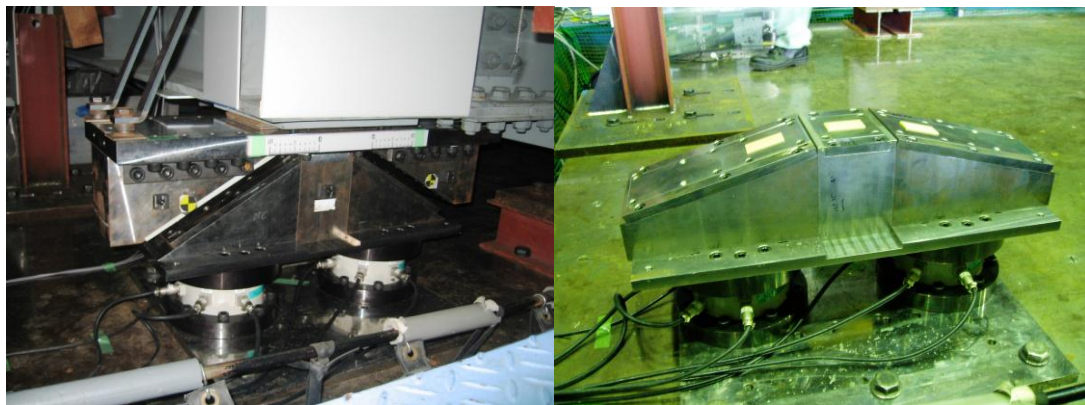
Figure 2.13 Uplifting Slide Bearing (UPSS)
