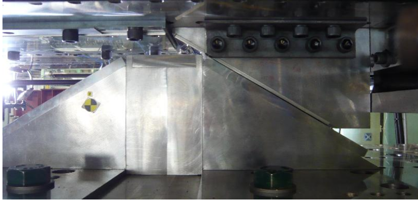
Figure 5.4 Test specimen with \theta=30^\circ during sliding
