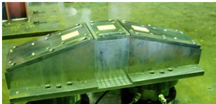
Figure 5.1 Lower component of the test specimen with PTFE pads
