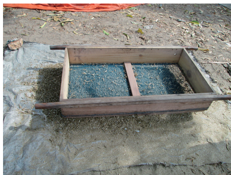
Photo 5. Sifter to separate fishmeal from dried dagaa (21/Feb./2013).
