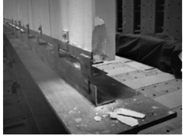
(b) Cracks and Spalling of Concrete at Panel Bottom
