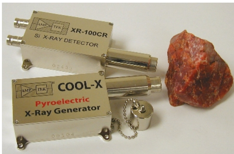
Figure 1.4. X-Ray emitter with pyroelectric crystal [10].
