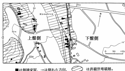
Fig.11. Locations of surface seismic fault, houses collapsed (■) and uncollapsed (□) in Kanehira, Gamagori city, Aichi prefecture, due to the 1945 Mikawa earthquake. Arrows denoted directions of collapse. After Ando and Kawasaki (1973).
