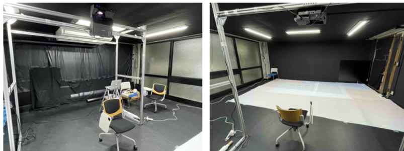
Fig. 3. Experimental environment (Left: Projector and its setting frame, Right: Projector and projection area).
