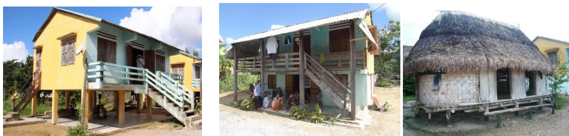
Figure 4.2. Provided house and adaptations: From left, original construction, modified stairs and balcony, modification of ground floor, traditional family house
