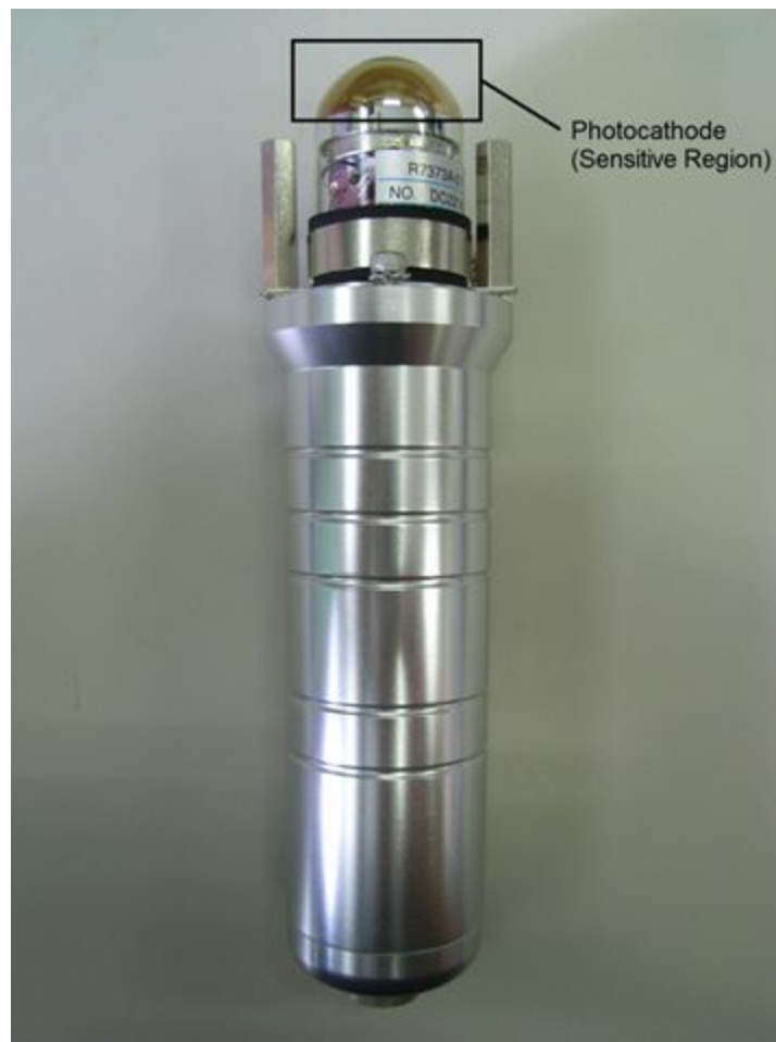
Figure 26. Photo of the PMT showing the sensitive region (R7373A-01; Hamamatsu Photonics Co. Ltd.).
