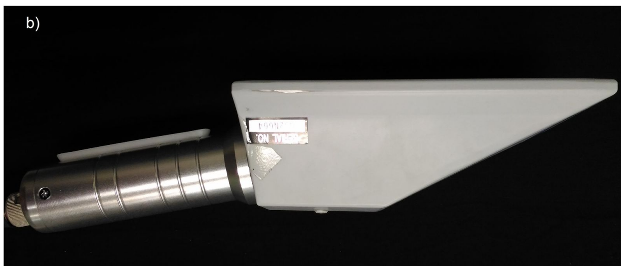
Figure 58. a) Schematic of the photocathode entry window to the sample sheet. b) Side view photo showing the angle of the PMT containing the photocathode.
