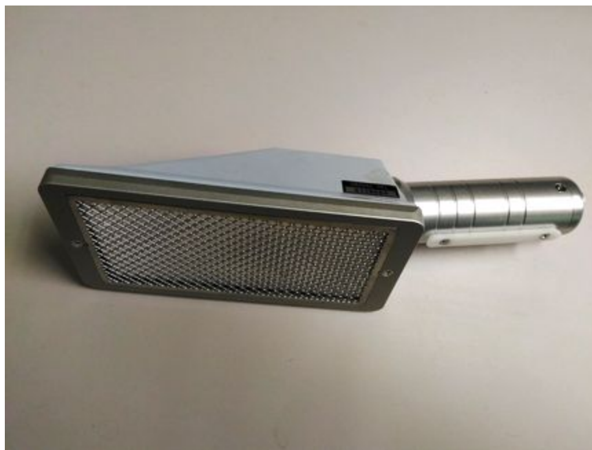
Figure 60. Photo of the detection section of a survey meter (OKEN - SPS210Z) using typical plastic scintillation material.
