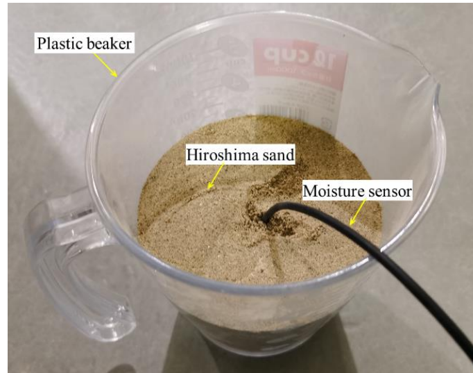
Fig. 3-33 Container for the calibration process
