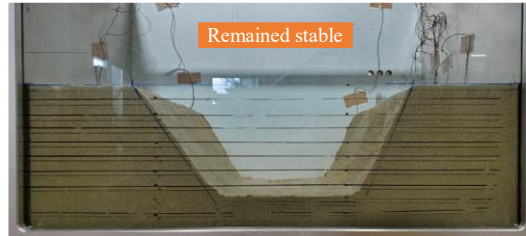
Fig. 4-30 Model state after centrifugal loading in Case 4
