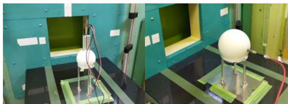
Fig. 1. BSS with a pair of lithium-glass scintillators (left) and BSS with a 6 LiF-shielded 3 He proportional counter (right).
