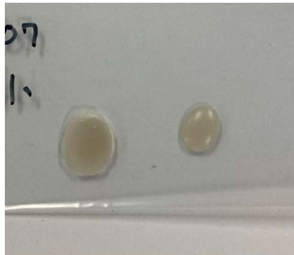
Fig. 1 Photograph of the fabricated transparent composite Li glass scintillator.
