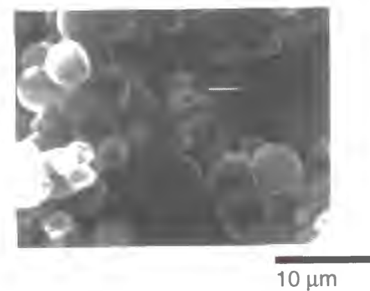
Figure 1-18 Scanning electron micrographs of lithium deposited on the as-received lithium foil electrode immersed for 72 h in in various electrolytes at 0.2 mA cm -2 (1.0 C cm -2 ), electrolyte ; PC containing 1.0 mol dm -3 (a) LiClO 4 , (b) LiCF 3 SO 3 , and (c) LiPF 6 .
