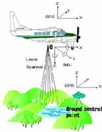
Fig. 4 Measuring principle of airborne laser scanning
