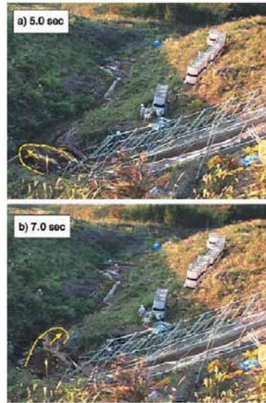
Fig. 20 Views of the debris flow resulting from the landslide fluidization between five seconds and seven seconds after failure.
