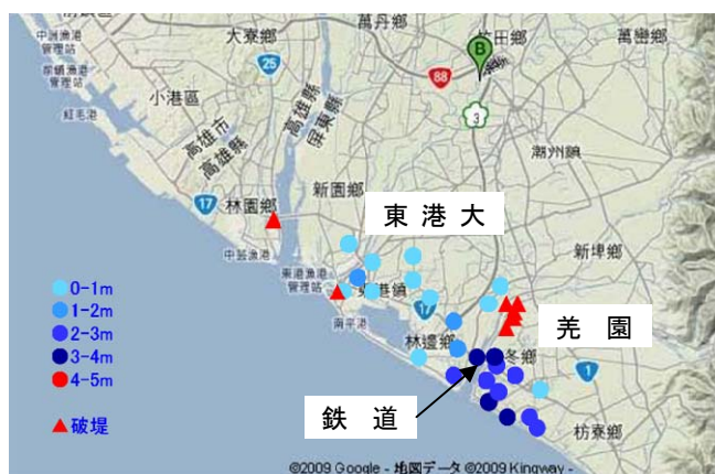
Fig.10 Inundation depth in Pingdong Country
