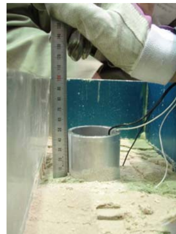
Fig. 5 Uplifted model manhole for CS4
