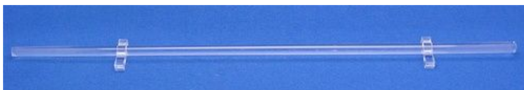
Fig. 6. Obtained fiber preform by extrusion method.
