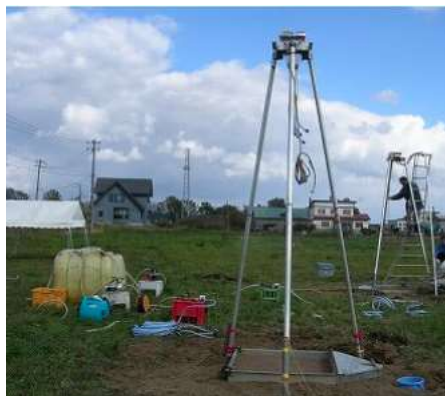
Photo 9 Field sprinkle equipment for infiltration
