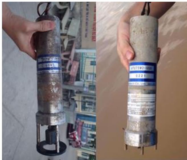
Figure 5.3 The installed turbidity meter (right) and salinity meter (left) in the VMD.
