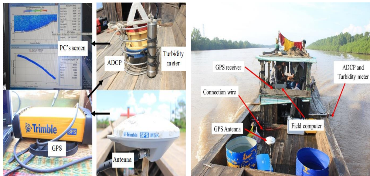
Figure 5.4 The measurement instrument used in the field survey.
