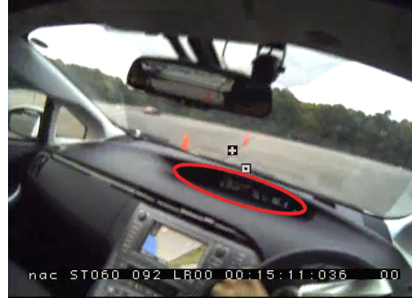
Figure 3.5: Driver's view as recorded by head-mounted camera. The part of the dashboard marked with an ellipse was used to estimate the head motion. Cross and square shaped markers are the tracked directions of the eyes.
