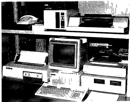
Photo. 11. Technical computer system for collecting the data of Tateyama and Suzaka, automatically. Data processing is also done by this system. (KAMITAKARA OBS.).
