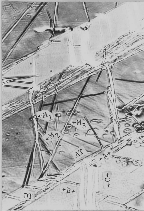
Photo.5.3 Microstructure of the Fe-25%Ni-0.7%C specimen which was deformed to 30% strain at 298K and cooled to 130K. Martensite(M 1 , M 2 and M 3 ) are considered to be formed from the annealing twin boundary(AT) on which deformation twins(DT) impinged. (x 930)
