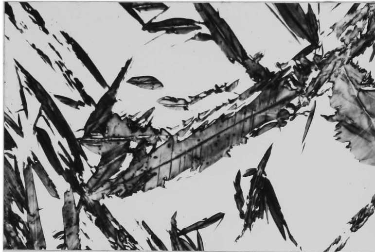
Photo.2.1 Optical microstructure of the Fe-29%Ni-0.2%C alloy strained 23% in tension at 247K. Etched by 35% \text{Na}_2\text{S}_2\text{O}_5 . (x 700)
