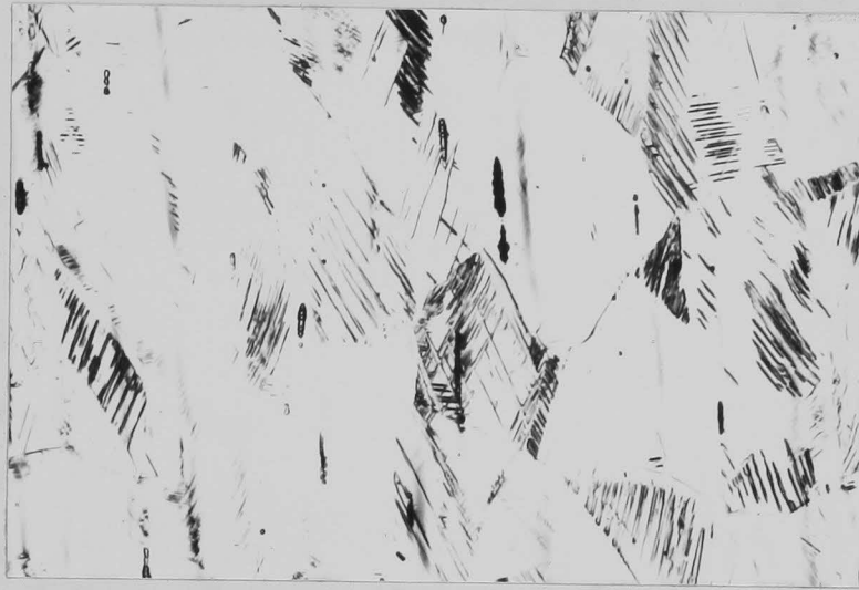
Photo.2.3 Optical microstructure of the Fe-32%Mn-0.2%C alloy strained 30% in tension at 77K. Etched by 5% Nital. (x 350)
