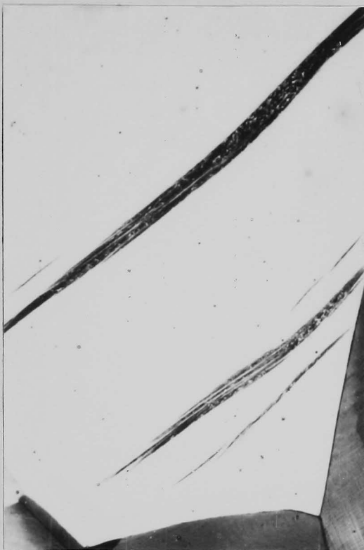
Photo.3.5 Optical microstructures taken from the Fe-23%Ni-0.5%C specimens deformed to about 30% strain in tension at 291K(a), 323K(b), 373K(c) and 473K(d), respectively, etched by 35% \text{Na}_2\text{S}_2\text{O}_5 solution. (x 700)
