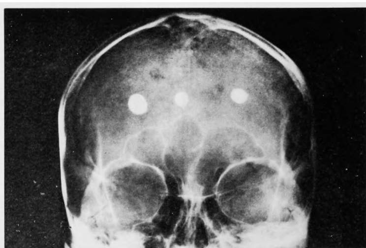
Fig. 7 The balloons were inflated with radiopaque, solidifying liquids. These liquids were sufficiently radiopaque for the balloon to be monitored under an X-ray image intensifier. The inflated balloons were placed on the forehead of a volunteer. Left : mixture of HEMA, ethyleneglycol dimethacrylate and metrizamide. Middle : mixture of HEMA, ethyleneglycol dimethacrylate and sodium iohalamate. Right : mixture of HEMA, ethyleneglycol dimethacrylate and meglumine sodium iodamide.
