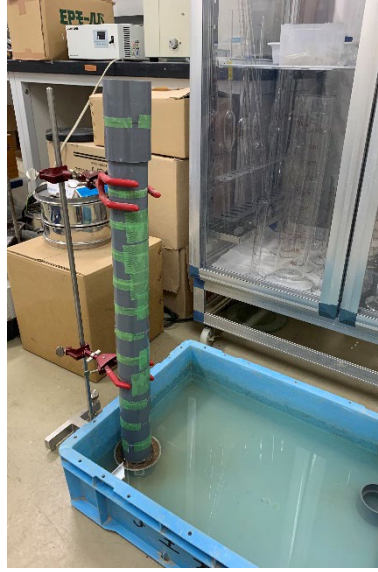
Figure 5.3: Schematic setup of the soil column method.
