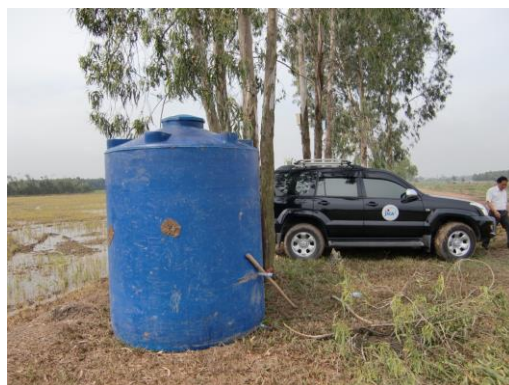
Figure 4-3 Storage tank of digested slurry
