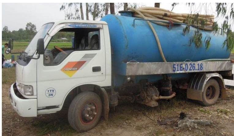
Figure 5-4 Photograph of vacuum truck
