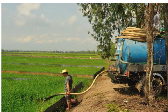
Figure 5-5 Application of digested slurry with the vacuum truck
