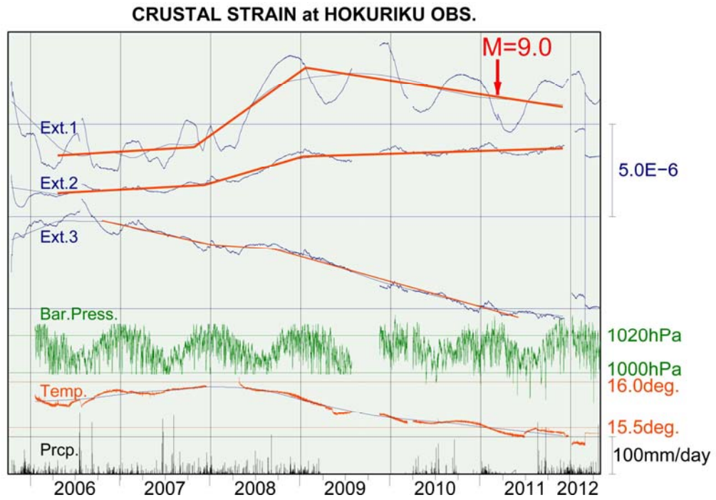
Fig.6 Ext.1, Ext.2, Ext.3 show the outputs of the extensometers. Blue : original data. Thin blue : average from extents for \pm 0.5 yr. Red: least mean square.
