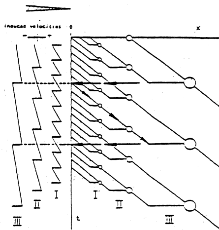
x - t diagram of an idealized pairing sequence of point vortices. The arrows show the feedback loop. For the pairings I through III the unsteady part of the induced velocity at x = 0 is plotted versus t (a positive transverse velocity is directed towards the high velocity side of the shear layer).
