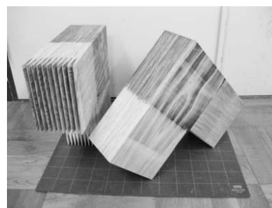
Figure 3. Developed joint method of compressed cross-lapped joint.
