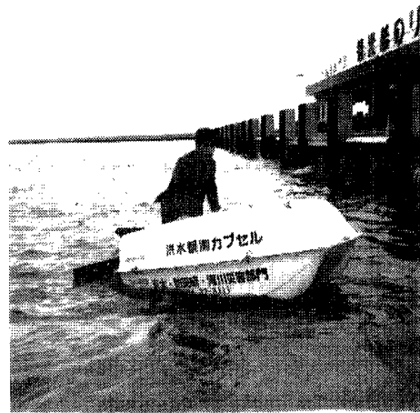
Photo. 5. A snapshot of the observation capsule tested in Lake Biwa.
