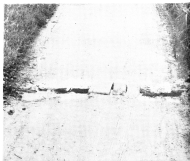
Photo. 11 A crossing ditch used in this test and the white line (by lime)
