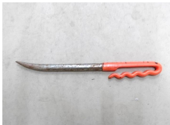
Fig. 12 Survey tool for riverbed softness
