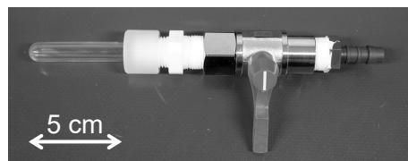
Fig. 2. Photo of the quartz container.
