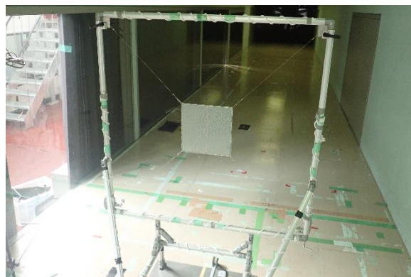
Photo 2 Photograph of the Jig supporting the Specimen
