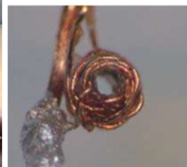
Mutual-inductance micro coil: 0.3 mm ID/1.0 mm OD.
