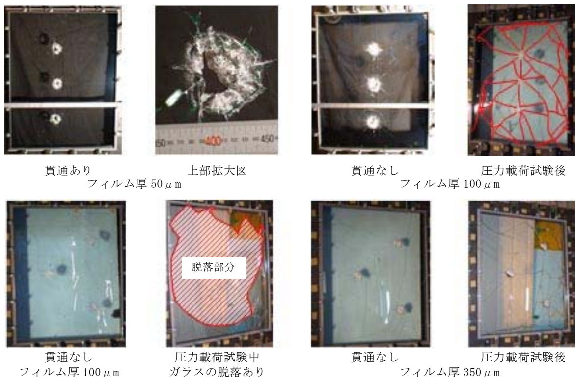
Fig. 18 Results of impact test of partially filmed glasses by missile type A
