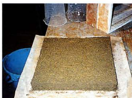
Bamboo-cement mat before pressing
