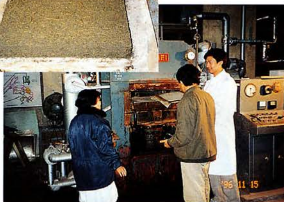
The rapid curing method of steam- injection pressing
