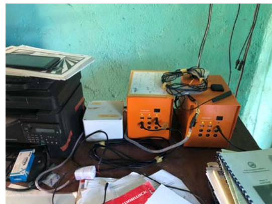
Photo 2 Measuring device installed in Vanuatu (White box is data logger and orange box is battery).
