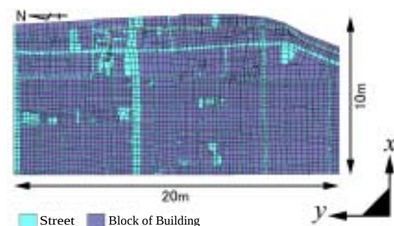
Fig.10 Meshes used in the calculation (entrances into underground space are not considered)
