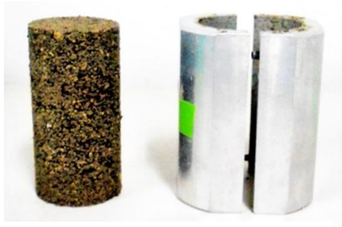
Photo 3.3 Mold used for specimen preparation
