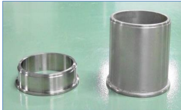
Photo 3.5 Consolidation ring with 20 mm (left) and 70 mm (right) height
