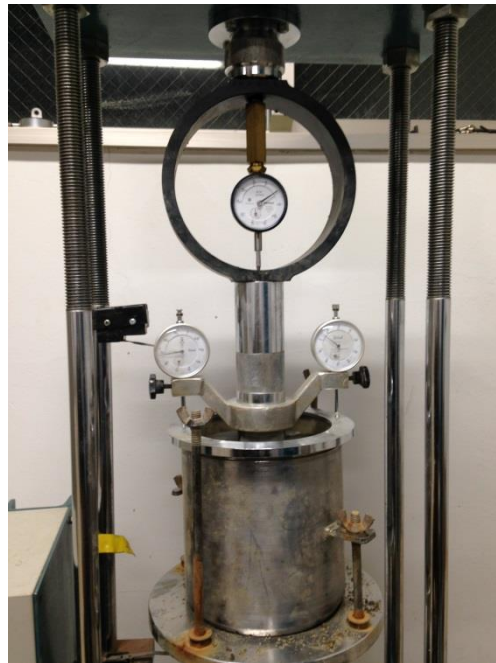
Fig. 3.14 CBR specimen with apparatus while taking reading
