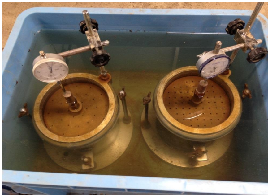
Photo 3.4 Specimens soaking by water
