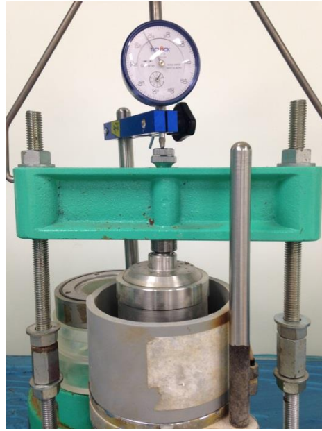
Fig. 3.15 Specimen at Oedometer apparatus while taking reading
