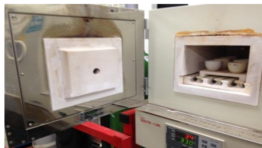
Photo 3.2 Specimen inside the muffle furnace
