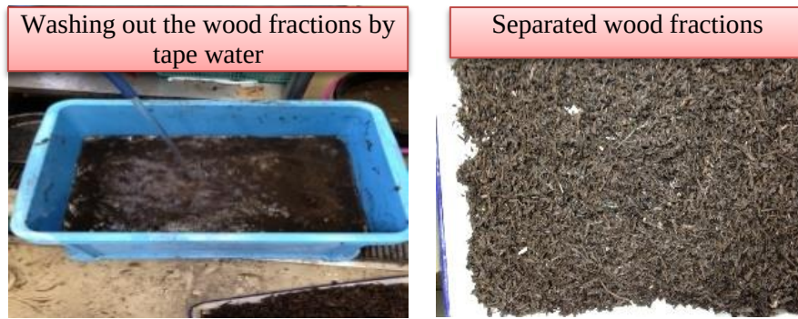
Fig. 3.1 Wood fraction separation from actual recovered soil
