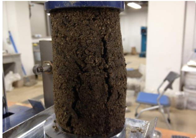
Fig. 3.10 Specimen while taking reading at unconfined compression test
