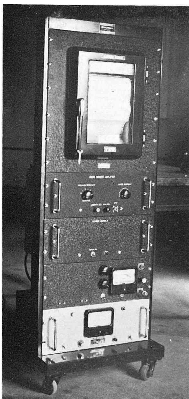
General view of the photometer head, the amplifier and the recorder
