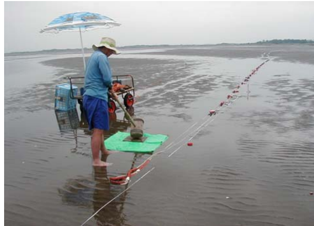
Figure 5.7.1. Surface-wave data acquisition using land streamer in tidal flat.
