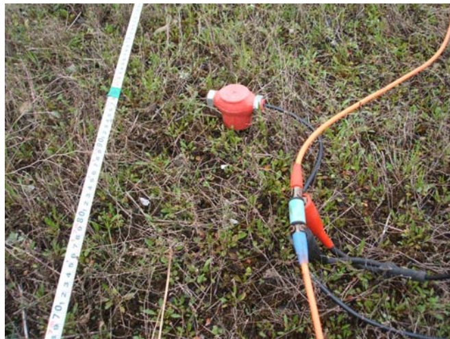
Figure 3.5.1. A sledge hammer (a) and a geophone (b) used in a surface-wave method.
