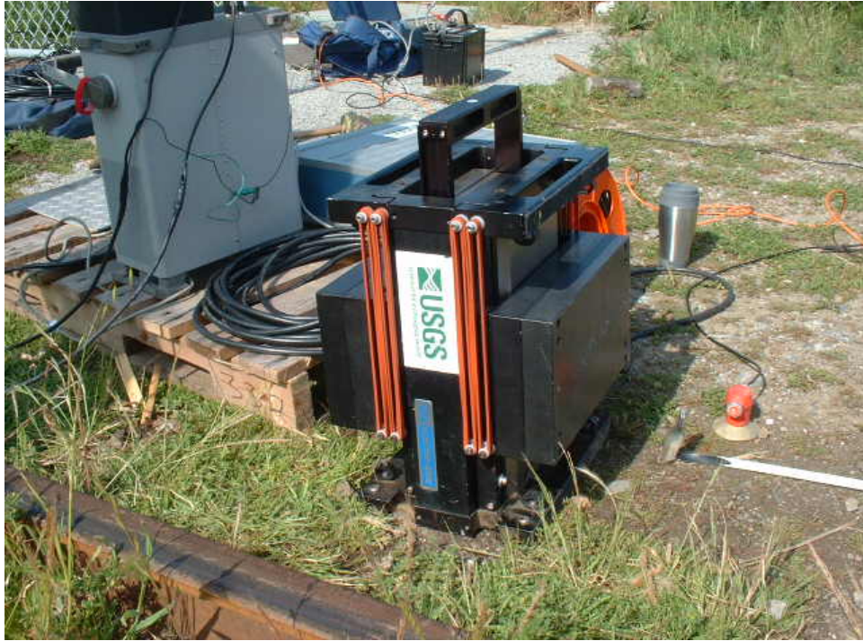
Figure 4.3.5 A typical shaker used in conventional surface-wave
