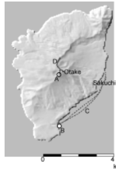
Fig.4 Map showing Suwanosejima. Observation points are A and B. Point A's name is 'Old Crater' and B's name is 'Kiriishi quay'. The measurement line of Tracerse method is C and D. The line C is measured by using a fishing boat. The line D is measured with walking Traverse.
