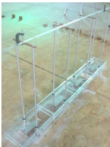
Fig. 7 Double barrier floating breakwater
