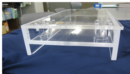
Fig. 2 Double barrier floating breakwater
