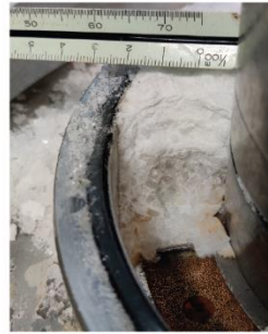
(b) A photo of an experimental shear zone in coarse halite particles (thick)
