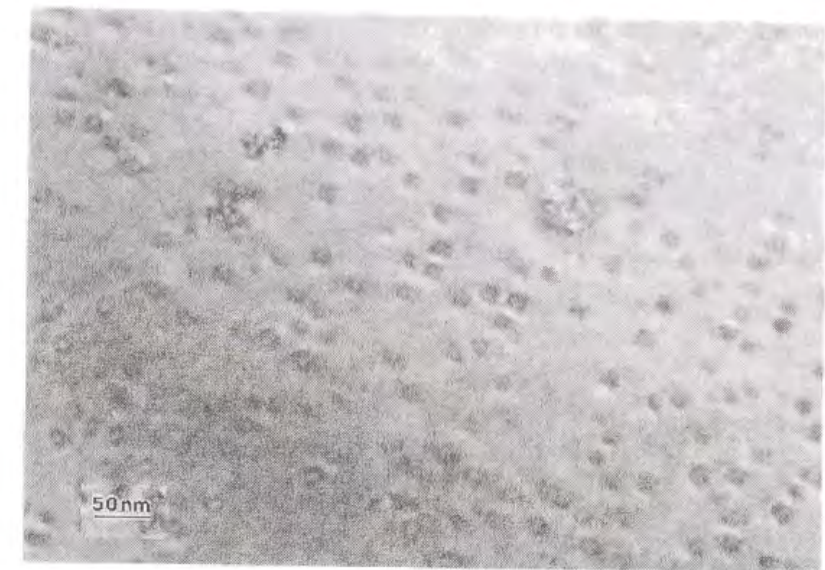
Figure 3-18 Plan-view TEM image of a sample grown by 10 cycles of an In-Ga-As sequence after supply of 2-monolayer In and As. Quantum dots having an in-plane diameter of 20 nm were observed.
