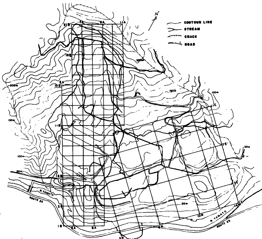
Fig. 1 A topographic map of the Kamenose landslide area. The systems of the measuring lines were established at intervals of 50 meters or 100 meters. They were also used as the horizontal coordinate systems.
