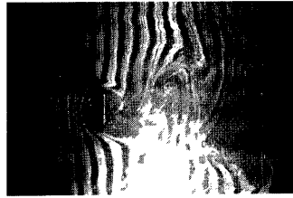
Photo. 2 Flow pattern around cylinder ( B/D = 0.5 , Re = 8.3 \times 10^3 , k = 2 S_t ).
